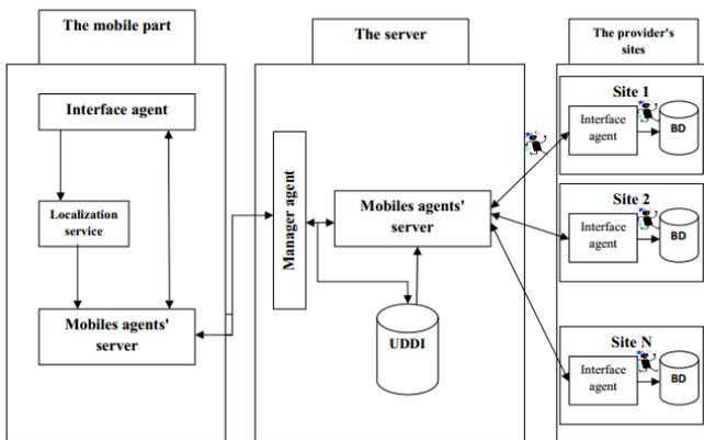
Figure 1. The overall system architecture.
